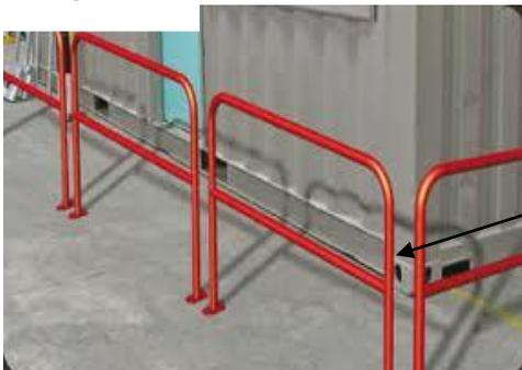
Ensure barrier gaps are present at each parking bay to allow pedestrian and wheel chair access to the centre pedestrian footpath as per Diagram 1 refer to AS2890 for dimensions and specifications.
